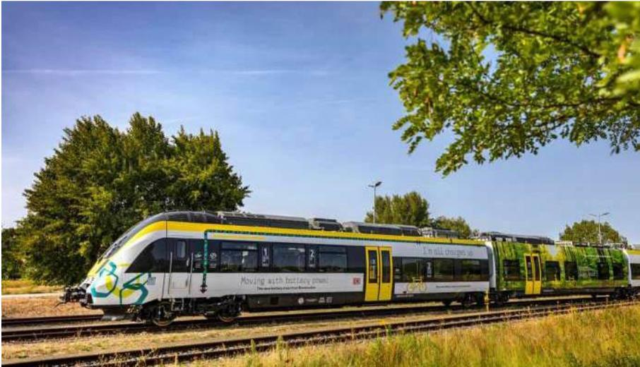
**Abbildung 20: Alstom Talent 3 BEMU (Battery Electric Multiple Unit)<sup>47</sup>**
